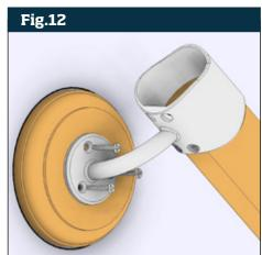
To fix rail for the bottom part of the stairs, offer the right hand end bracket onto the end of a handrail. Pilot drill through bracket screw holes using 3mm dia drill bit and secure using screws supplied (Fig.13).
